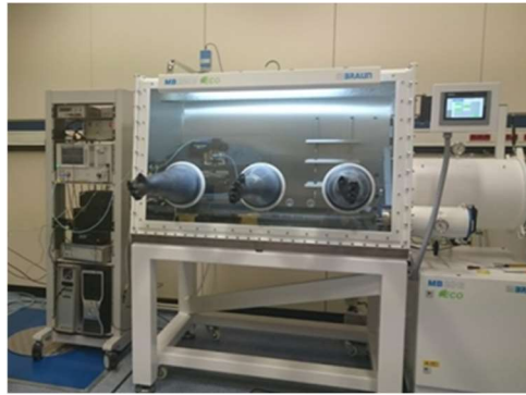
Figure 2. SMM setup at LNE, where the AFM part is located in a glove box.
