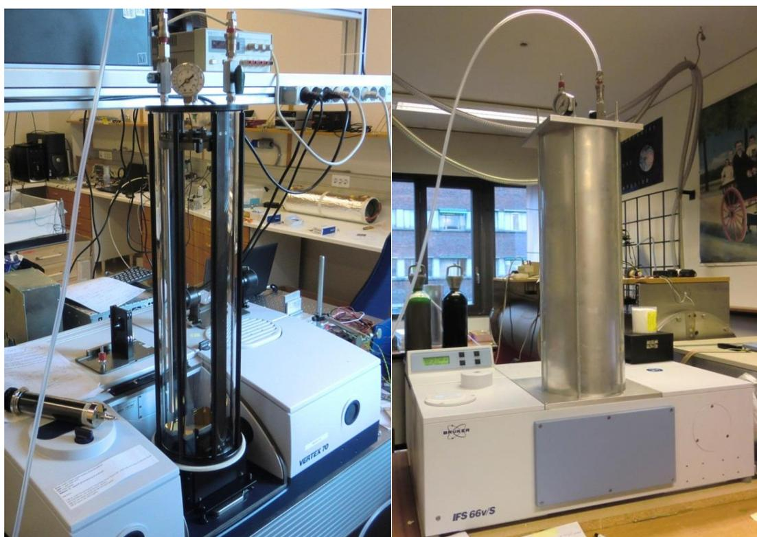
*Figure 6: 35 m cell mounted on Bruker Vertex 70 (left) and Bruker IFS 66v/S operated under vacuum (right). Pictures taken with permission from [10].*
