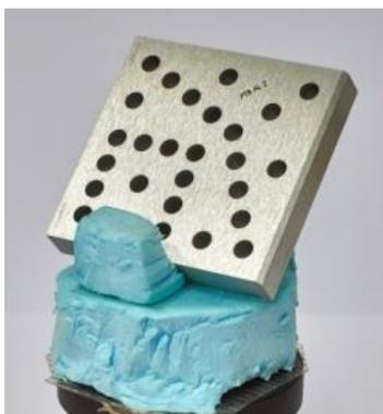
Fig. 27. PTB/NMIJ aluminium hole plate.
