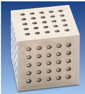
Fig. 31. PTB titanium calotte cube for testing industrial CT systems.
