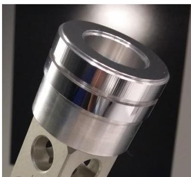
Fig. 28. Multi-wave standard made of Al designed by UFSC/CERTI (courtesy of UFSC/CERTI).
