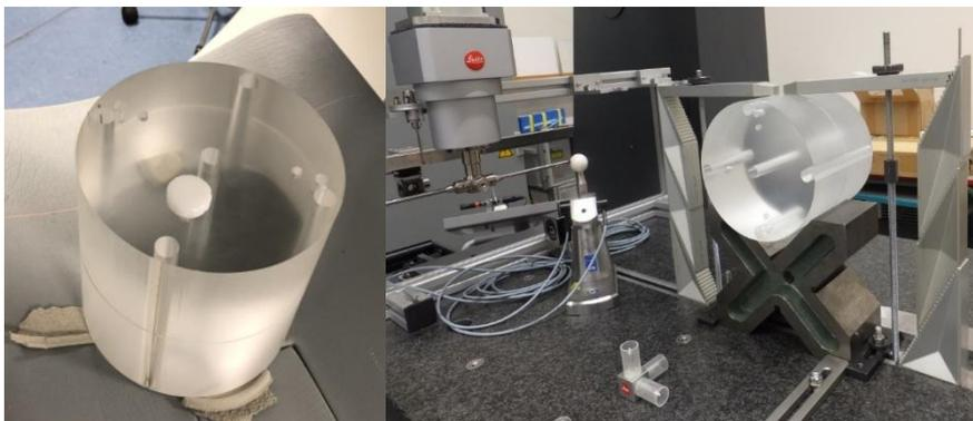
Fig. 8. (Left) CTDI-Phantom used for the study; (right) CTDI-Phantom mounted in a tactile CMM for the reference measurement.
