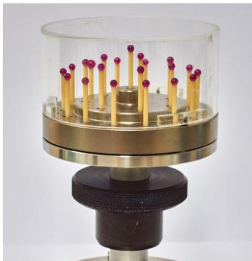
Fig. 11. Multi-sphere standard (22 spheres) manufactured by Carl Zeiss, Oberkochen, Germany.
