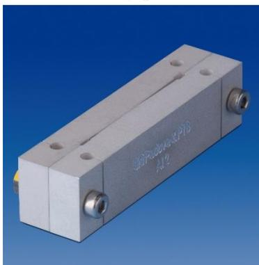
Fig. 33. PTB/University Padova (Al&Al) CT gap standards for testing industrial CT systems.
