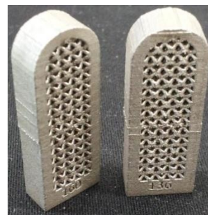
Figure 42: Lattice specimen produced by LNE/ NIST with intended missing struts made of CoCr alloy
