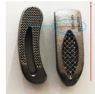
Figure 22: Shrinkage on a spinal implant built in the direction \vec{z}
