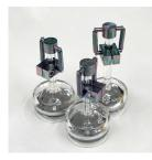
The results also show that the filter system, to produce mercury free air, is working properly. Furthermore, and most importantly, the system is producing a flow with a stable mercury vapor content.
