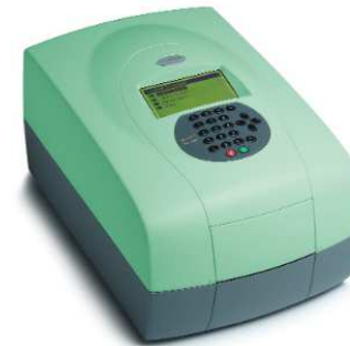
Deepwell plate reader (405 and 630 nm)
