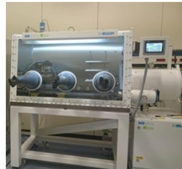
Figure 2. Glovebox at LNE, where the AFM part is located inside.
