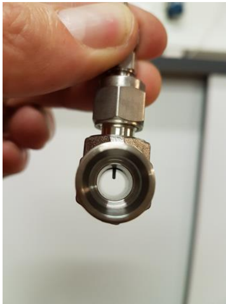
Figure 38 – Photo of the thermocouple measuring the gas temperature at the entry of the mass flow meter (1 mm diameter thermocouple type K).
