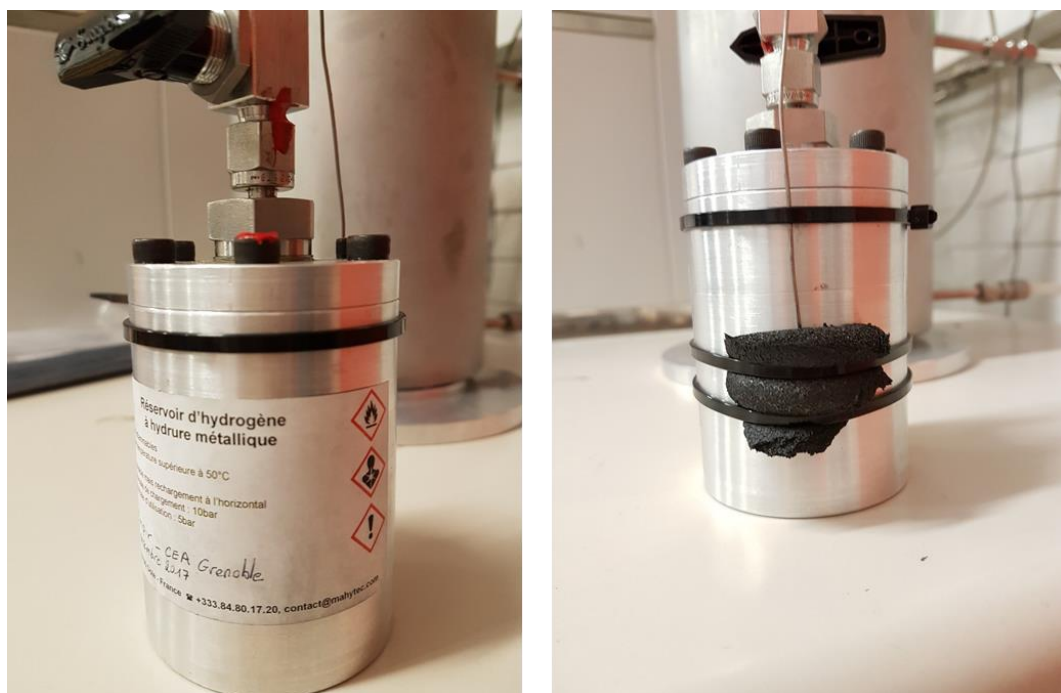
Figure 39 – Instrumentation of the tank. The thermocouple is installed under isolating neoprene foam, in order that the measure is closer to the temperature of the container wall than the temperature of the thermal fluid.
