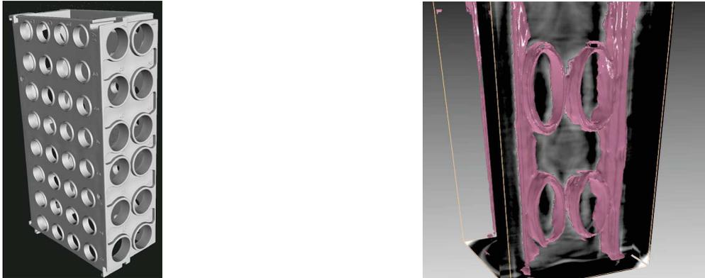
Figure 16: Visual comparison of the reconstructed volume (a) 8 mm sphere by XCT, (b) 8 mm sphere by THz-CT; (c) polymer beak holder reconstructed volume by XCT and (d) beak holder by THz-CT at 2.5 THz.
